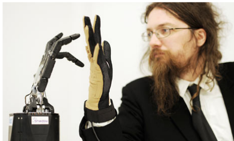
Rich Walker of Shadow Robot Company with a robotic hand that could be used by army bomb disposal personnel. Photograph: Ben Stansall/AFP/Getty Images
